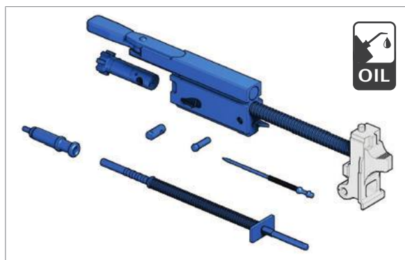
Fig. 117: Lubrication points of functional elements
